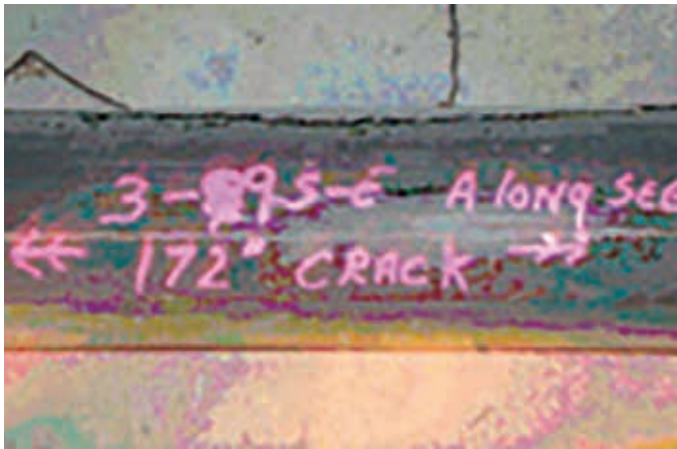
Cracked HDPE Duct
