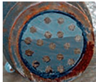
Result of void grouted with Vacuum Grouting
