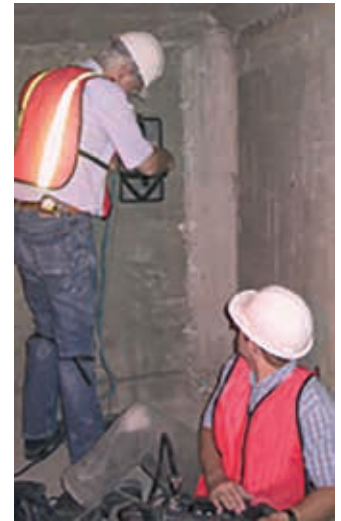
Using Impact Echo to locate voids in the tendon
