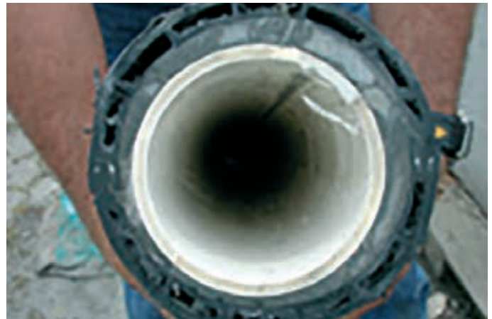
Simulated Repair of Cracked HDPE (White Pipe) duct using Half Pipe (Outer black Pipe). Annulus between pipes has been grouted.
