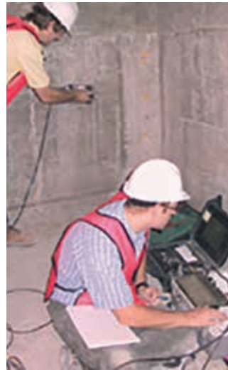
Locating tendons using GPR
