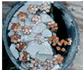
Result of void grouted with conventional methods
