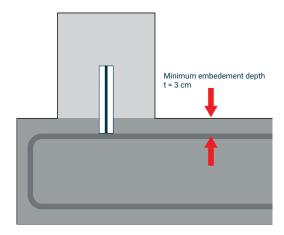
All joints between the metal waterstops are to be fixed with the separate formbraces type K23 or Fixing Clips type K23.
