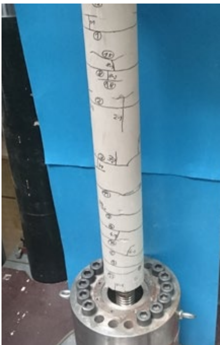
DYWI® Drill Hollow Bar grout column crack width analysis
