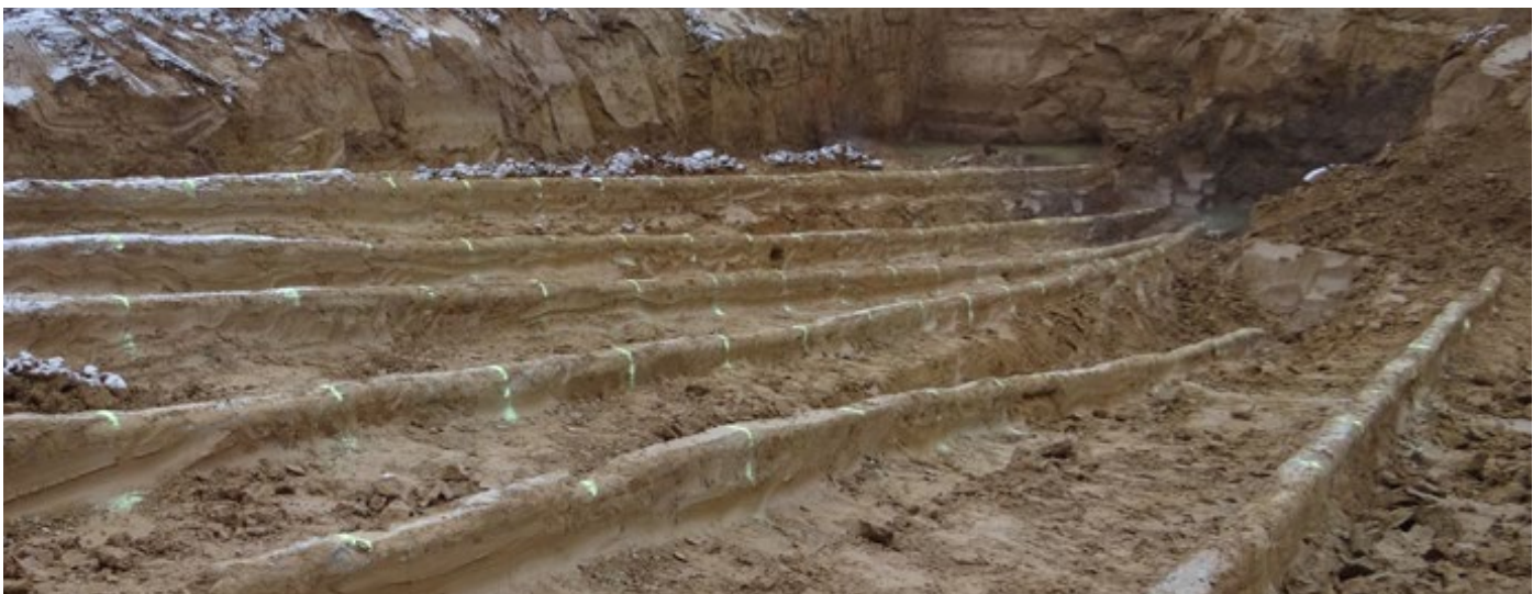
Research & Development - DYWI® Drill Hollow Bar drilled into sand and exhumed to measure the diameter and consistency of grout cover
