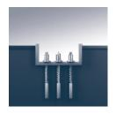
Uplift occurs in a large variety of foundation structures independent of the existing water level or by variable superimposed loads. The bottom slab of construction excavations (underwater concrete or high-pressure injection slabs) must be secured temporarily during the
