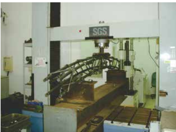
Lattice Girders Testing
