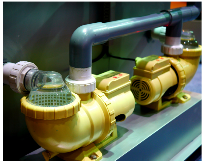
Electric motor with onboard controls.
