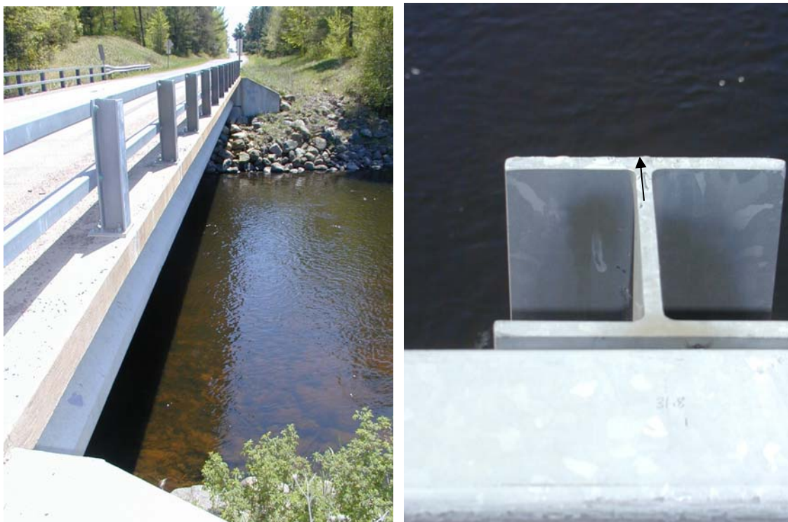
Figure 15. Namekagon River at Earl flow monitoring site photos. A) View along river cross-section from right bank, looking at the left bank (i.e., facing south on North Road). B) Close-up view of bridge railing benchmark used for measuring stage, or distance of water surface below benchmark. Benchmark (marked by arrow) is located at upper edge of I-beam column located 31.8 ft from the left bank edge-of-water.
