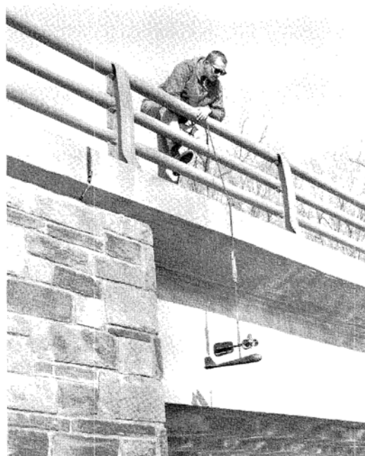
Figure 4. Cable suspension system: A) USGS handline, and B) example of handline, attached to flow meter and Columbus weight, in use from a bridge.
