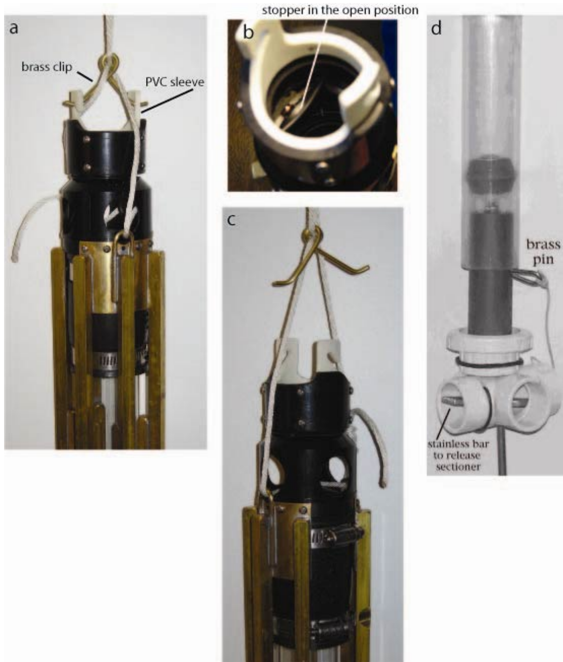
Figure 1. The Wiegner surface corer. a) The corer in the set position, ready to be deployed. b) When deploying the corer, the black stopper must be in the open position, resting against the black rubber band. c) The corer being retrieved from the sediments (brass clip has been released from the white PVC sleeve, and the line has been pulled taut, allowing the black stopper to close. d) The sectioner with the brass pin in place.
