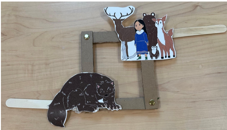
Parallel Motion Device With 4-Bar Linkage
