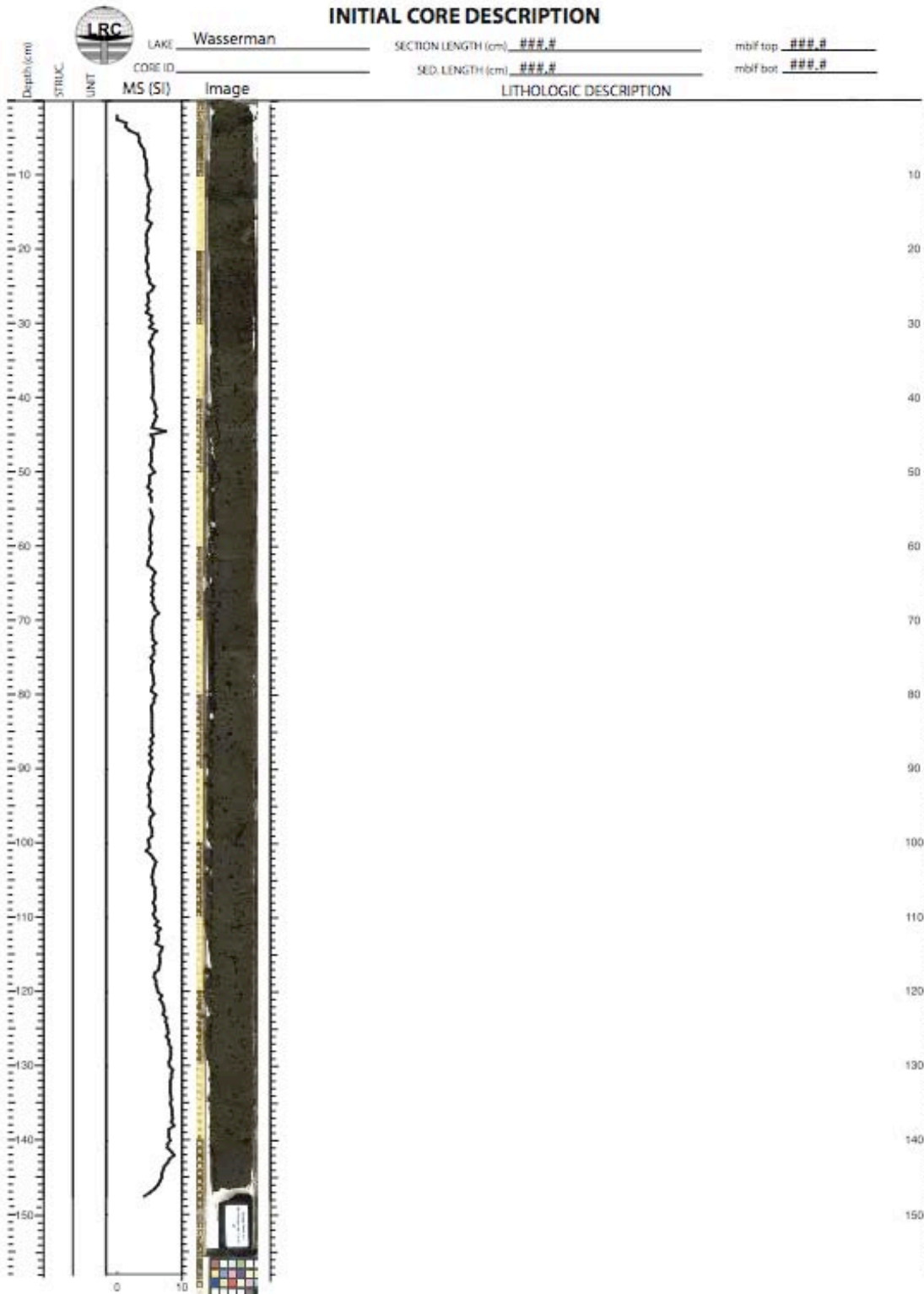
Figure A-10. Magnetic susceptibility and core scan, Wasserman Lake core. Field extruded to 28 cm.
