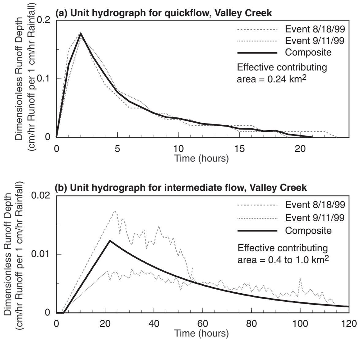
**Figure 6.--Unit hydrographs for quickflow and intermediate flow at mouth of Valley Creek, 1999**
