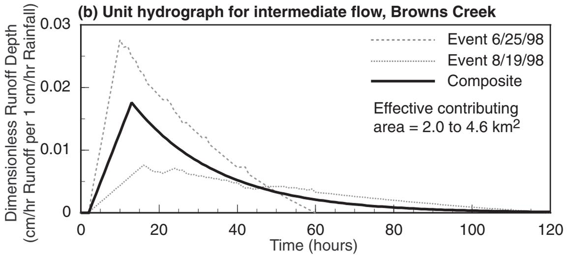
**Figure 7.--Unit hydrographs for quickflow and intermediate flow at mouth of Browns Creek, 1998**
