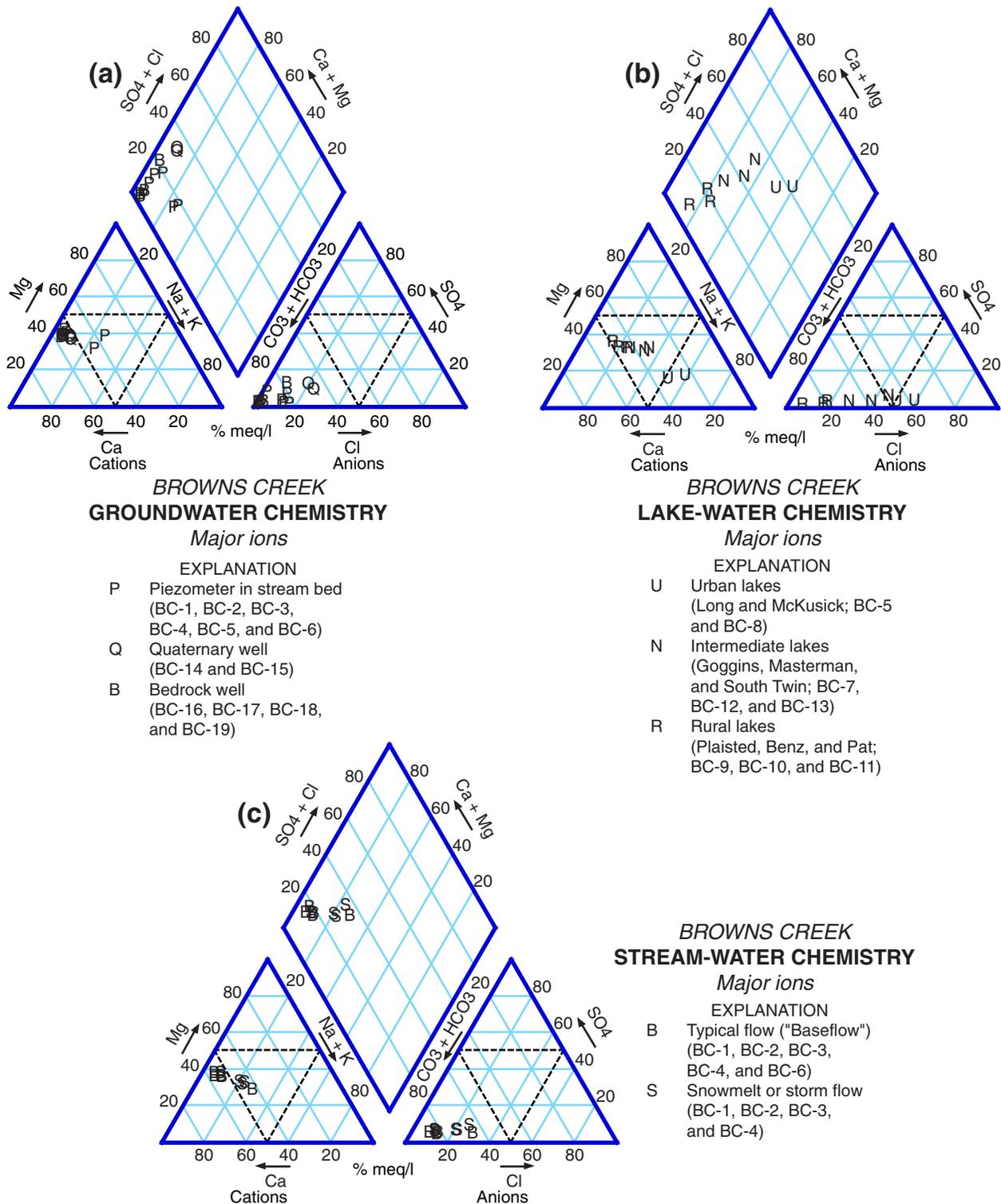
**Figure 16.--Major ion chemistry in the Browns Creek Watershed: (a) groundwater, (b) lake water, and (c) stream water.**
