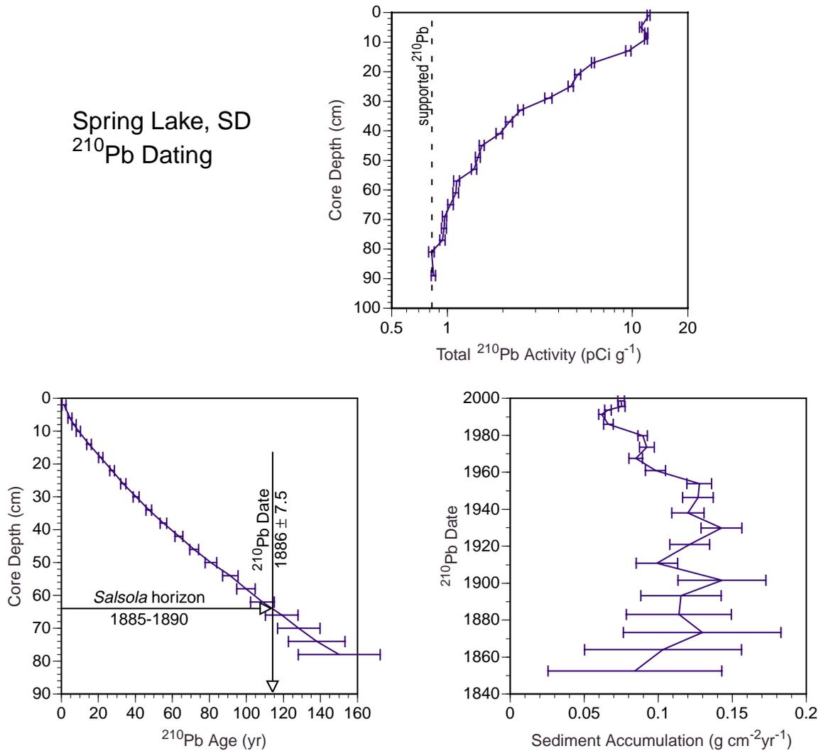
**Figure 9.** Lead-210 activity profile for the Spring Lake surface core and the resulting age/depth profile and sediment accumulation rates determined by the constant rate of supply (c.r.s.) mode; error bars represent  $\pm 1$  s.d. The depth at which Russian thistle (*Salsola iberica*) first appears in the pollen record corresponds to a <sup>210</sup>Pb date of 1886; Russian thistle spread throughout Day County between 1885 and 1890 (see text.)
