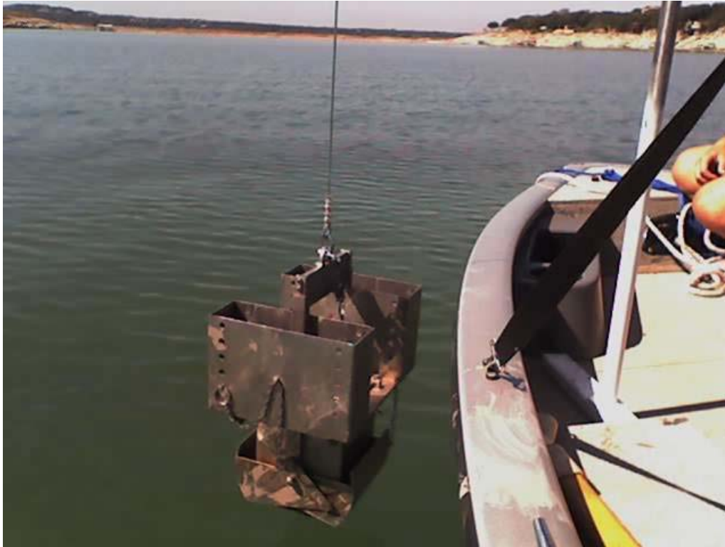
Figure 11. Wildco Model 191-A12 box corer with liner deployed for recovery of sediments for push cores (photos by R. Kiesling USGS).
