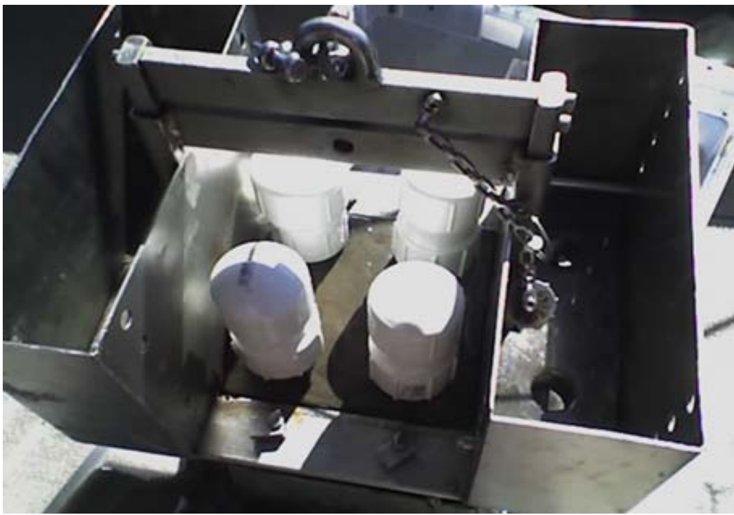
Figure 12. Wildco Model 191-A12 box corer with push cores (photos by R. Kiesling USGS).
