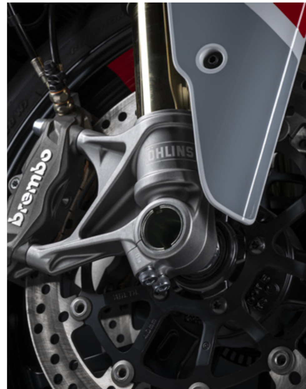
1 Fully adjustable Ø 48 mm Öhlins fork with TiN treatment.
