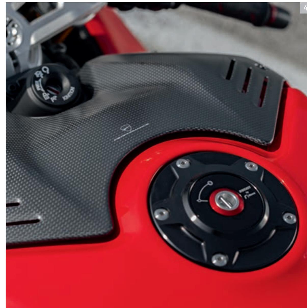
4 Carbon tank cover. Billet aluminium tank cap
