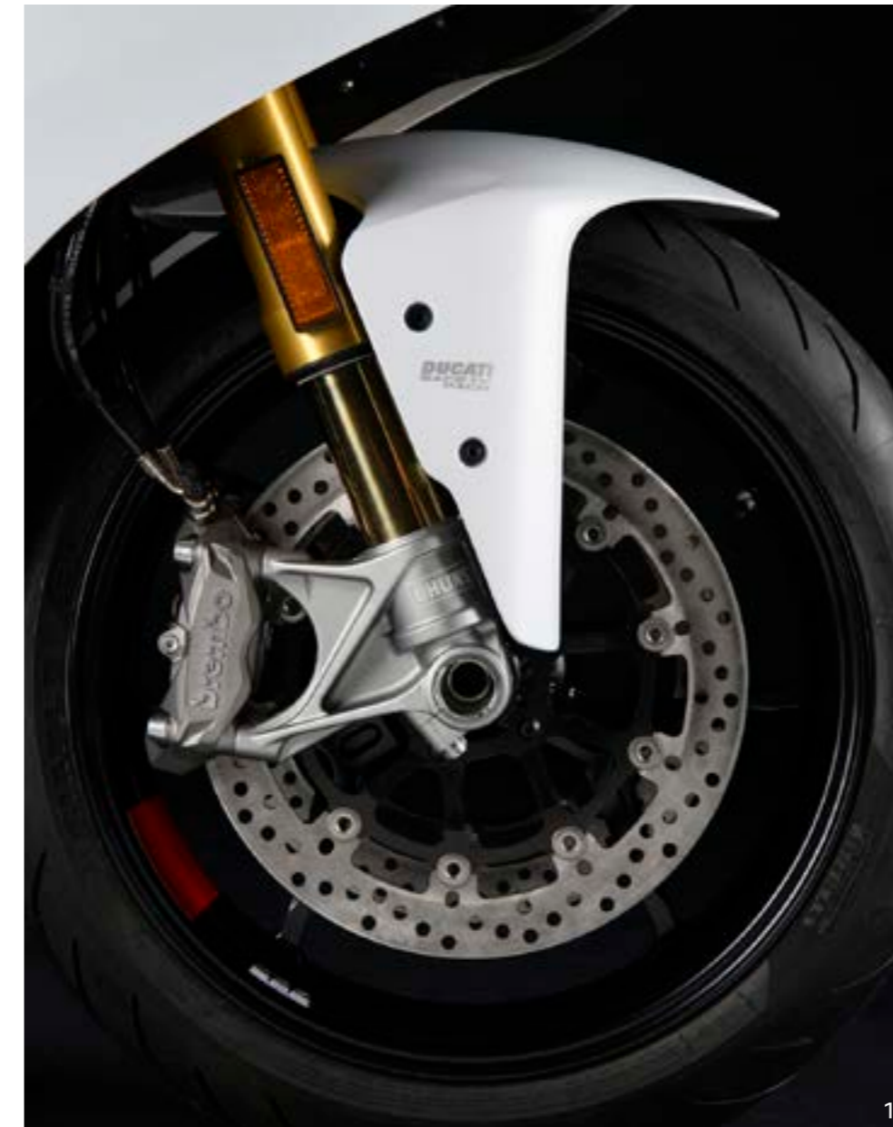
1_ Fully adjustable Ø 48 mm Öhlins fork with TiN treatment. 2_ Fully adjustable Öhlins monoshock with integrated gas tank. 3_ Passenger seat cover.
