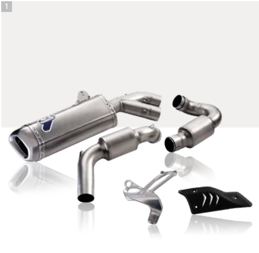
1 Complete racing exhaust with titanium silencer
