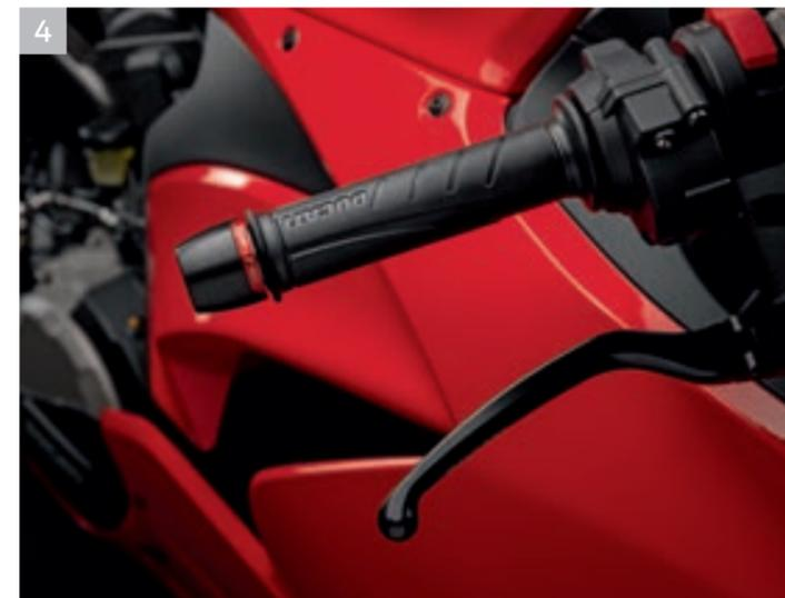
4 Billet aluminium handlebar balancing weights.
