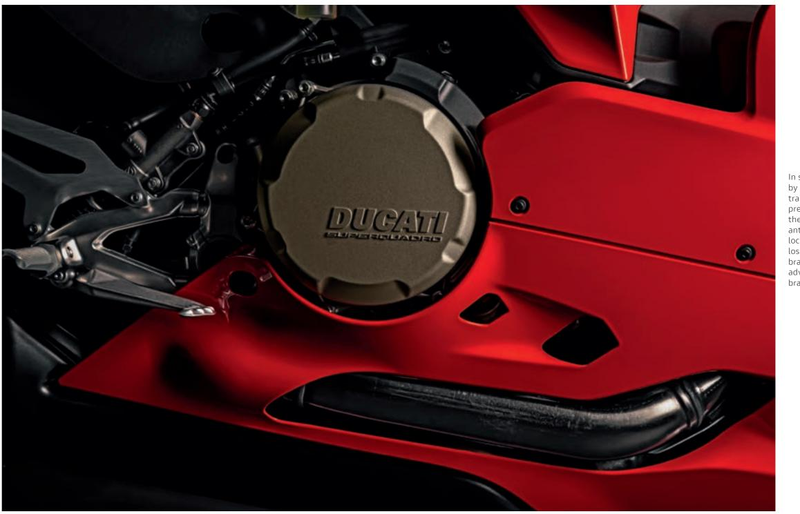
In sports riding conditions, characterised by aggressive shifting and engine brake transfer, the same mechanism reduces pressure on the clutch discs, allowing them to work in the racing-derived anti-wheelie mode, which obstructs any locking of the rear wheel and subsequent loss of rear stability during aggressive braking, while offering the additional advantage of excellent modulation when braking.
