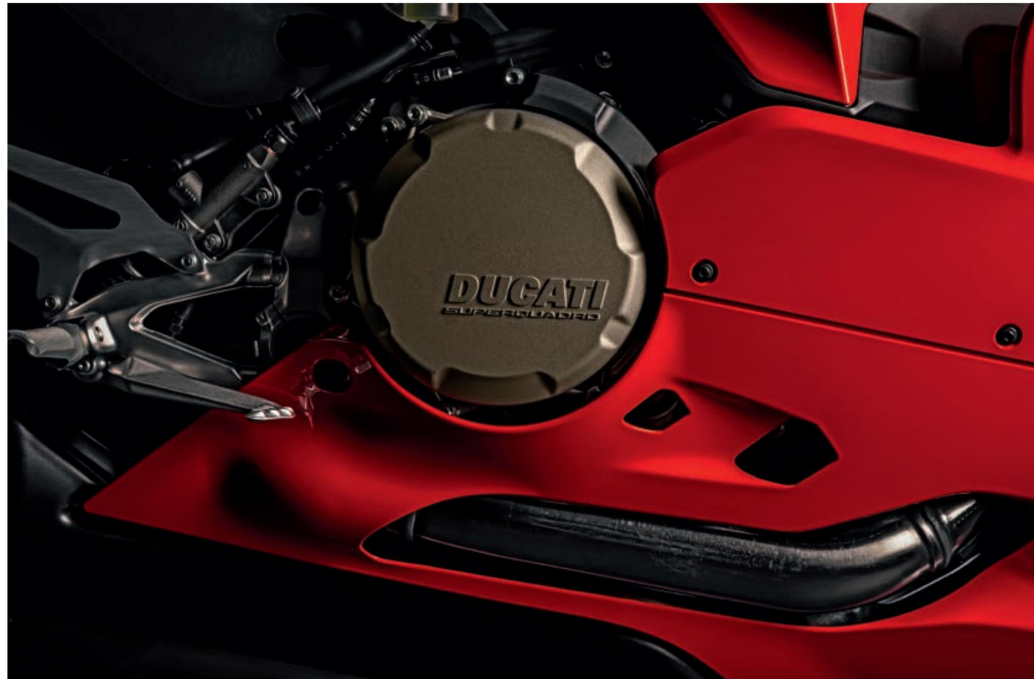
In sports riding conditions, characterised by aggressive shifting and engine brake transfer, the same mechanism reduces pressure on the clutch discs, allowing them to work in the racing-derived anti-wheelie mode, which obstructs any locking of the rear wheel and subsequent loss of rear stability during aggressive braking, while offering the additional advantage of excellent modulation when braking.
