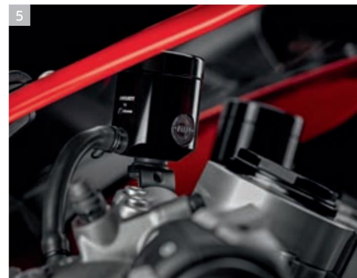
5 Brake fluid reservoir. Clutch fluid reservoir.
