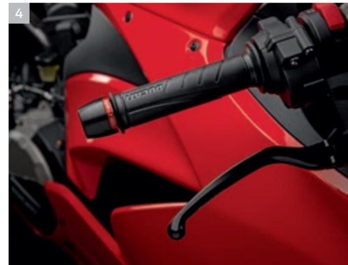
4 Billet aluminium handlebar balancing weights.
