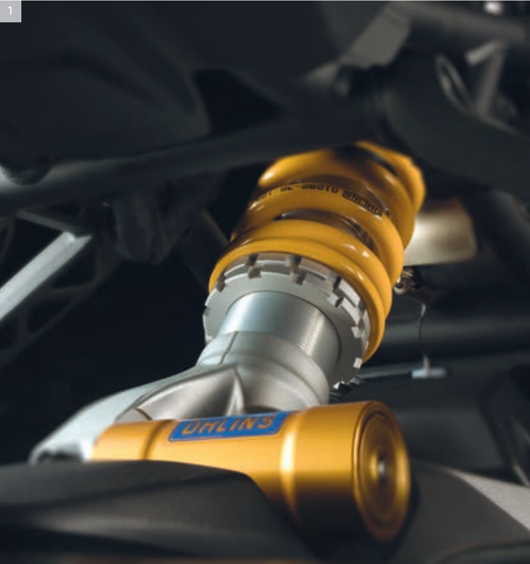
1 Fully adjustable Öhlins front and rear suspension
