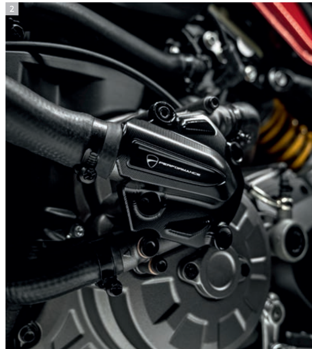
2 Billet aluminium water pump cover
