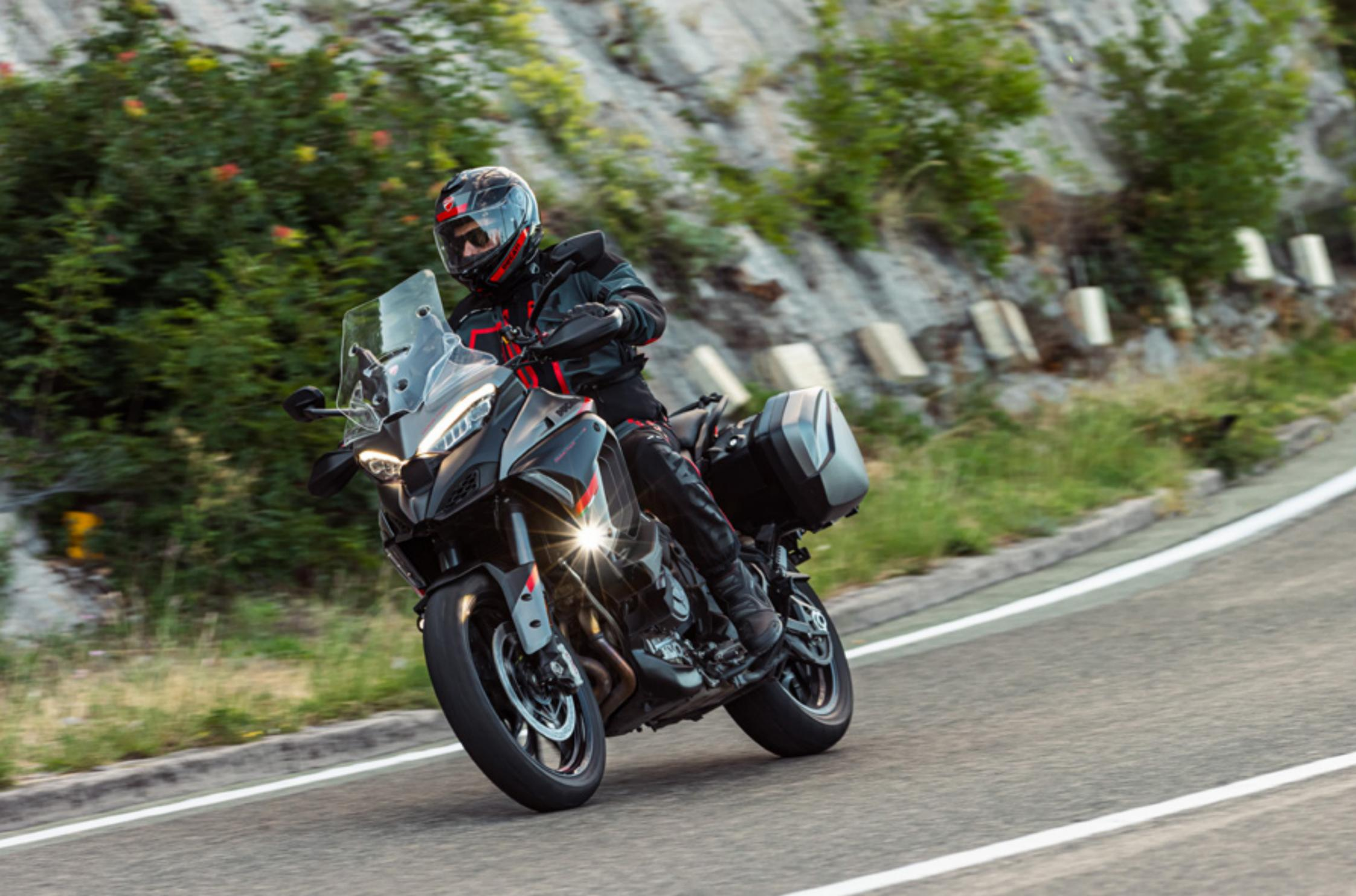
The 19" front wheel ensures a round, easy and intuitive ride in all conditions, guaranteeing the precision and responsiveness required by sports riding. To ensure the possibility to fit spoked rims, the Multistrada V4 S Grand Tour is equipped with a new generation double-sided swingarm, an object with a unique design, developed by applying additive technology, which offers the perfect balance between compactness, stiffness and lightness.
