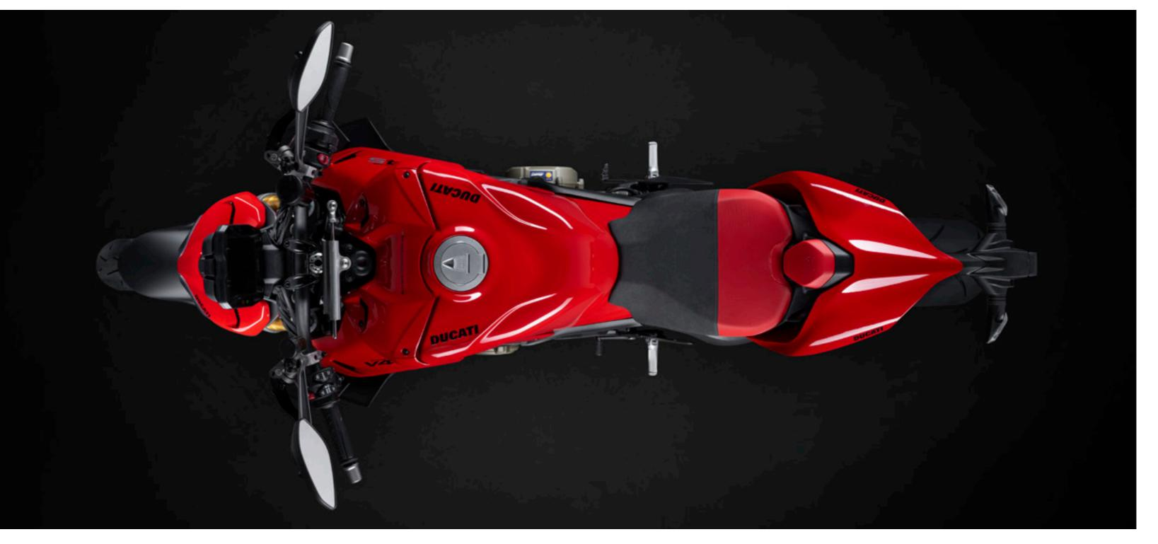
cornering. Compared to the Panigale V4, the tank has been suitably modified in the lower area to allow the fitting of a saddle with more foam to increase rider comfort. As with track bikes, the tank has a portion of its capacity located under the rider's seat. In the front, the space not occupied by the fuel has been used to place all the electronics, including the battery.
