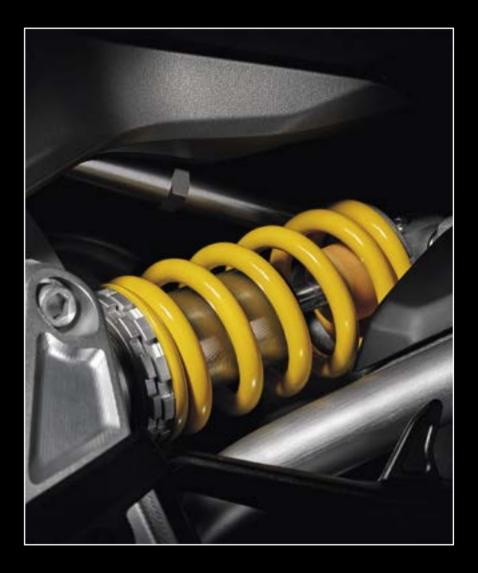
The XDiavel has a completely adjustable 50 mm front fork with black anodised outer tubes and DLC coating (on the S version). At the rear, an adjustable damper with a remote reservoir is mounted in an nearly horizontal position and works together with a progressive linkage. In addition, both the front and rear suspension have been updated to ensure even greater comfort without sacrificing precision or effectiveness.
