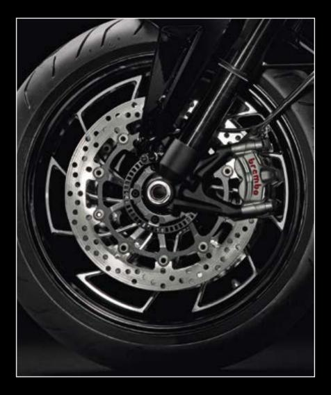
The XDiavel is equipped with a Brembo braking system with Bosch Cornering ABS as standard equipment. Front braking performance is ensured due to two 320 mm semifloating discs, radial Brembo monobloc 4-piston callipers with radial master cylinder. At the rear there is a 265 mm disc with a 2-piston floating calliper.
