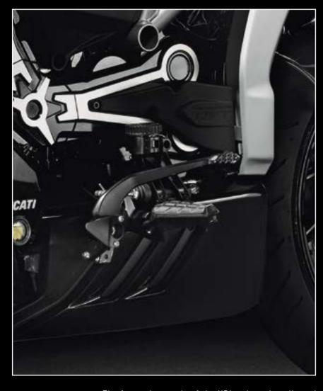
The forward controls of the XDiavel can be adjusted in three positions. A central footpegs kit and a rearward footpegs kit are available as optional accessories, both can be further adjusted to ensure the best ergonomic positioning for every rider.
