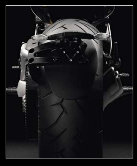
The imposing rear tyre, 240 mm in width, boasts doublecompound technology to increase grip during extreme leaning.
