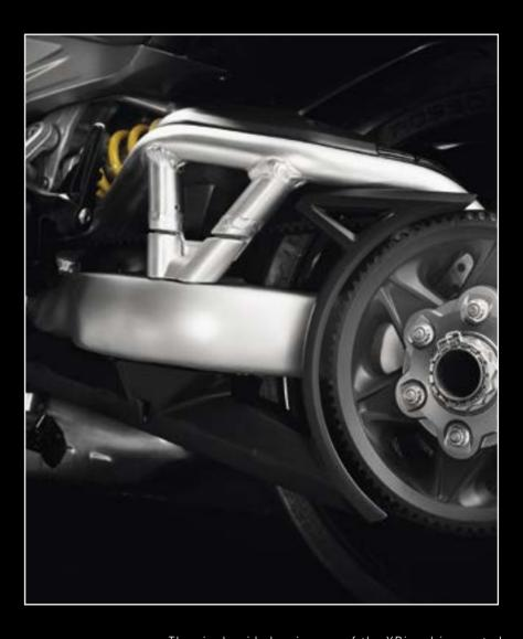
The single-sided swingarm of the XDiavel is created by combining three different technologies within the same component. The lower part is cast while the upper is composed of a tube trellis and an extractable forged element that allows for the transmission belt to be replaced.
