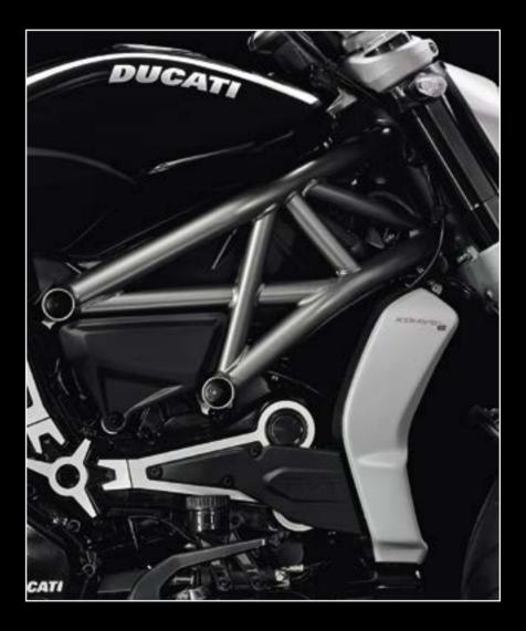
The XDiavel frame is a steel trellis frame linked to the engine heads that becomes a stressed element of the chassis.
