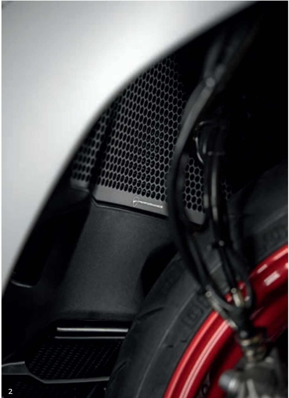
2_ Protective mesh for water radiator. 3_ Aluminium number plate holder.
