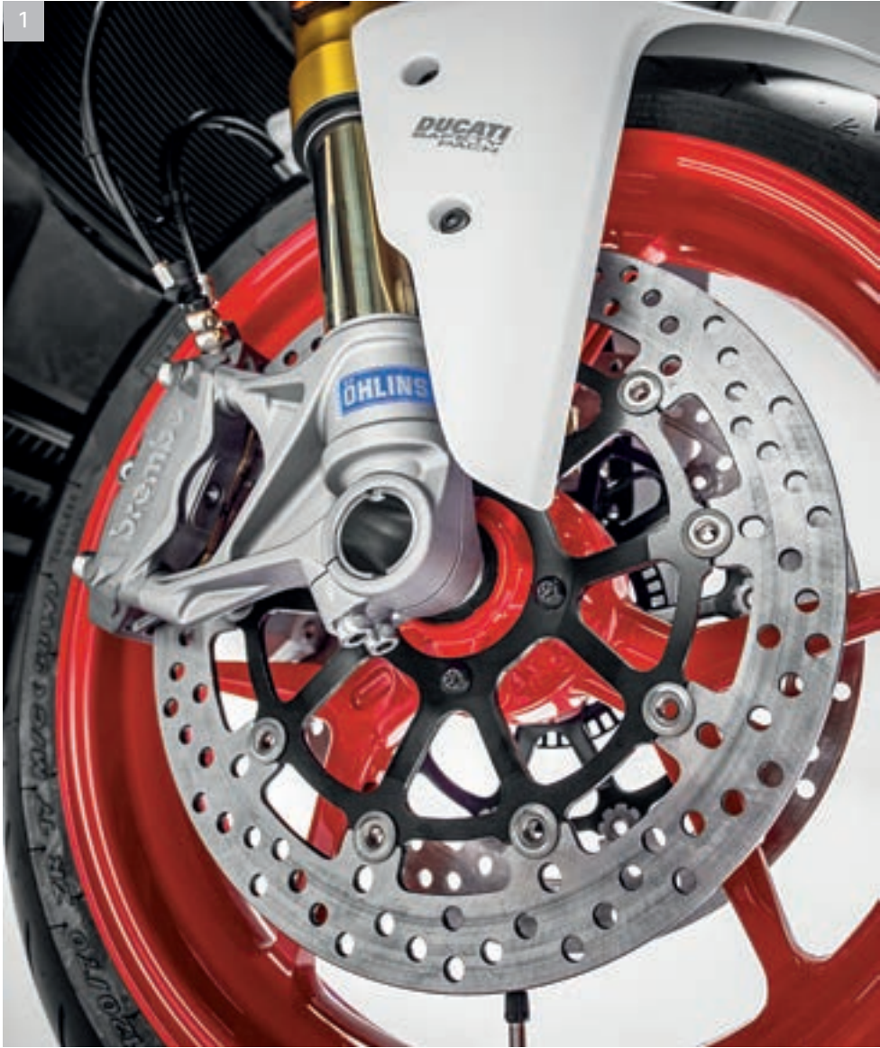
1 Öhlins fully adjustable fork, 320 mm discs and radial caliper Brembo monobloc.
