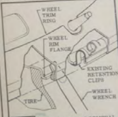
FIG. 2 WHEEL TRIM RING REMOVAL
