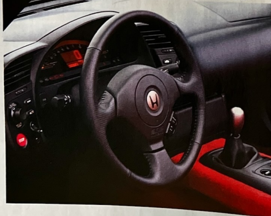
■ The view through the fat 3-spoke wheel reveals a half-moon bar-graph tach, a large digital speedometer display and smaller horizontal readouts for coolant temperature and fuel level.
