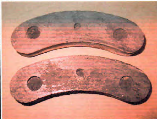
Burnt pads, material is flaking off
