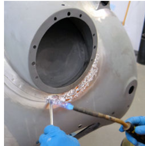
Applying the first of approximately 50 lbs of lead
