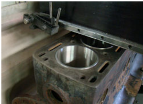
Surgacing block after installation of new liners
