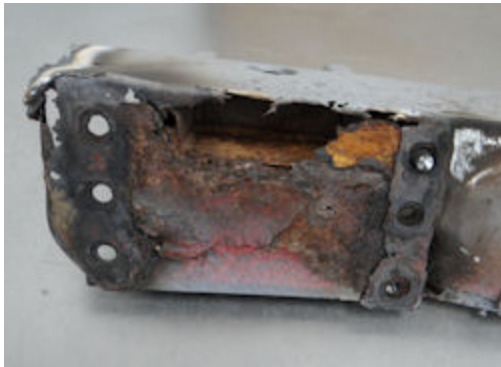
Back side of LH rocker panel where it attaches to the A pillar
