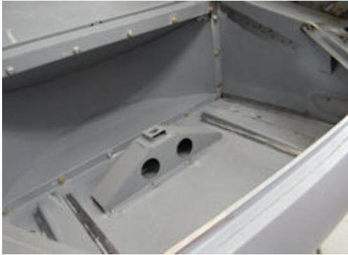
Trial fitting spare wheel well and hold-down bracket
