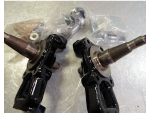
Front suspension components have been powder coated
