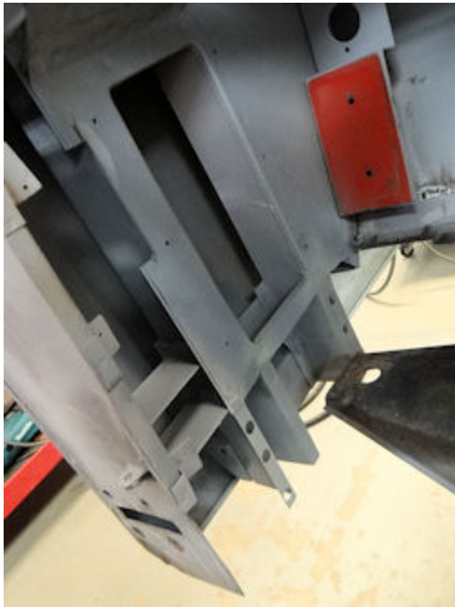
Inner A post now reconstructed
