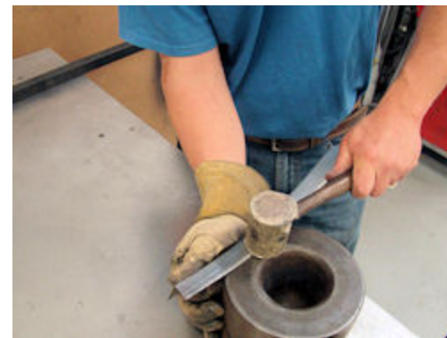
Hammering the flange into shape
