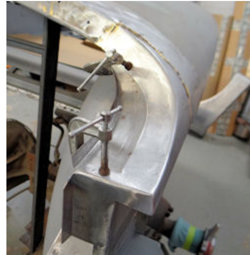
About to weld the various upper panels together
