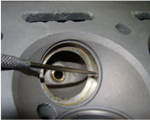
With the valve seat removed, the step above the seat is clearly visible
