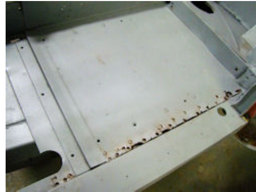
Drilling out spot welds to remove floor section
