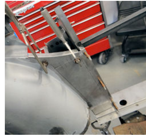
Ready to weld B pillar sections in place
