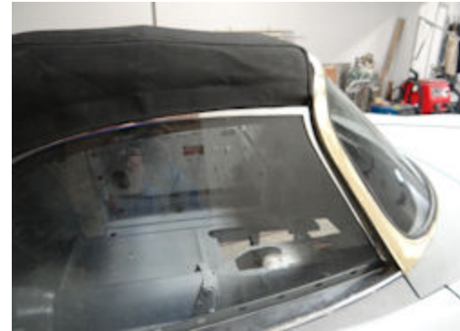
Trial fitting and adjusting the convertible top frame
