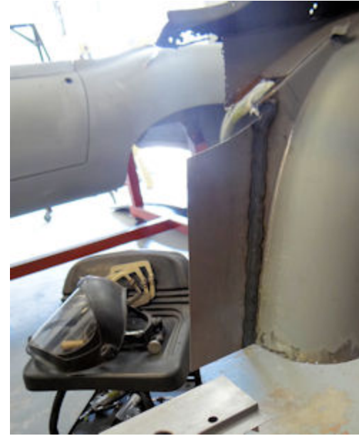
Beginning to reconstruct B pillar
