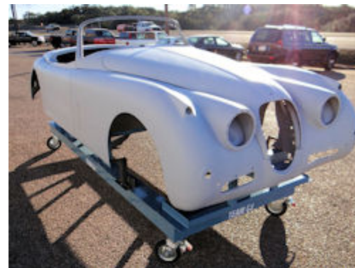
All of the bodywork has now been completed and the car has been primed
