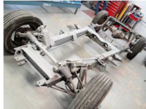
Chassis will be disassembled, blasted, repaired as needed and powder coated
