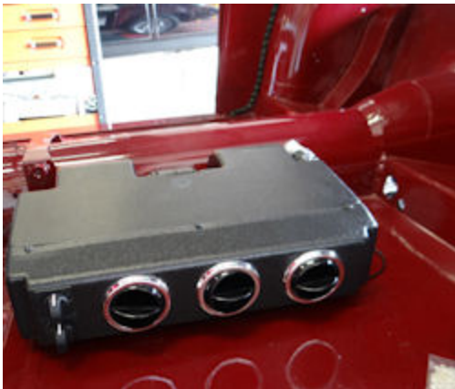
AC unit will be centrally mounted beneath dash
