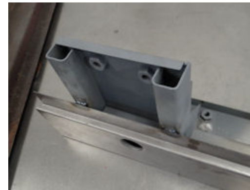
Welding securing bracket to LH rocker panel
