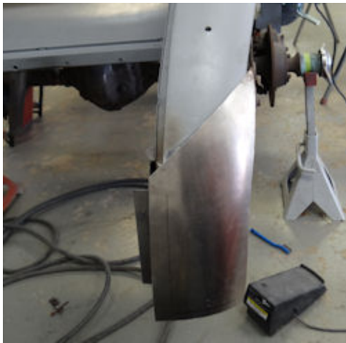
Trial fitting replacement panel
