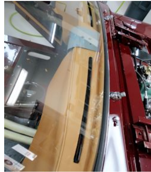
Hide dash top carefully trimmed around demister vents
