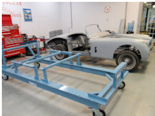
Time to put the body on the frame jig
