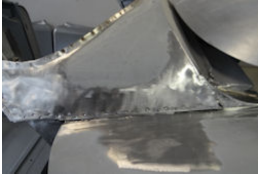
About to lead load the right side cowl
