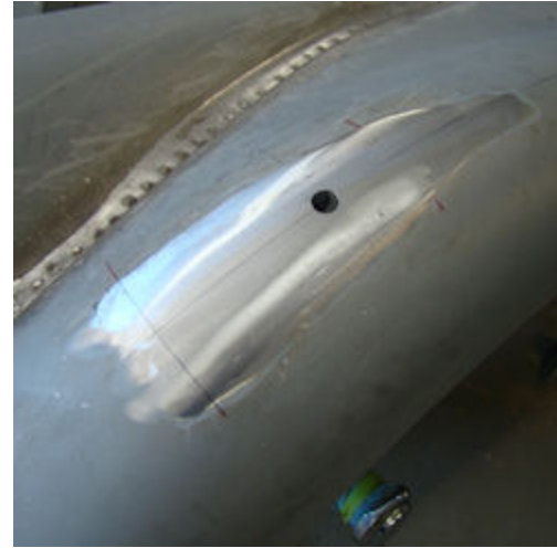
Hole cut in new panel for marker light harness
