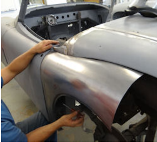
Trial fitting rear wing repair panel
