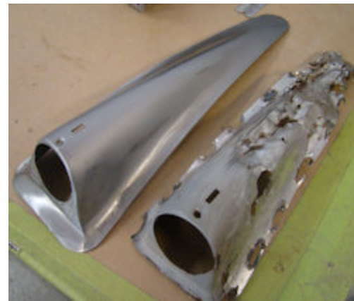
Replacement marker pods differ slightly from originals and will have to be modified
