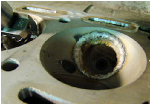
Most of the valve seat pockets had to be welded up and re-cut
