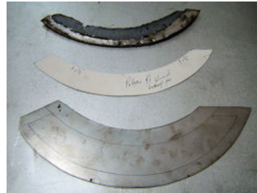
Repair panel being fabricated from new sheet metal
