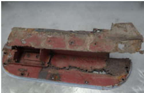
What is left of the driver's "B" shut face panel
