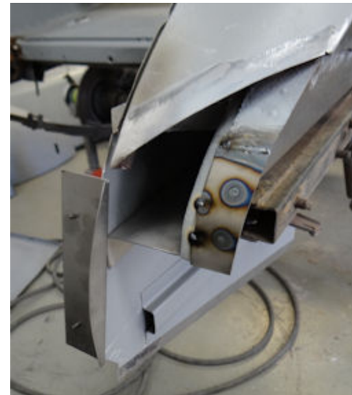
Panel is first reconstructed internally
