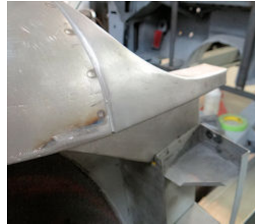
Repair panels now welded in place
