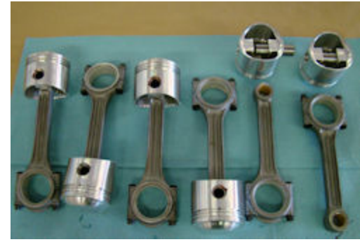
CJ forged pistons hung on rebuilt rods
