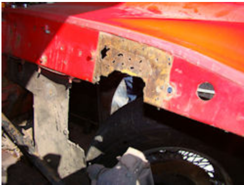
There are a number of places that will require sheet metal repairs, although nothing too serious
