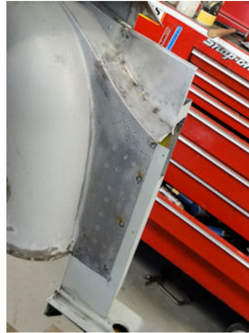
Upper and forward panels now welded in position
