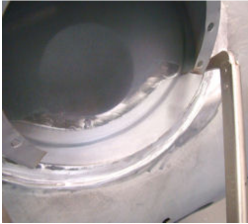
Repair panel for top surface of wing clamped in place
