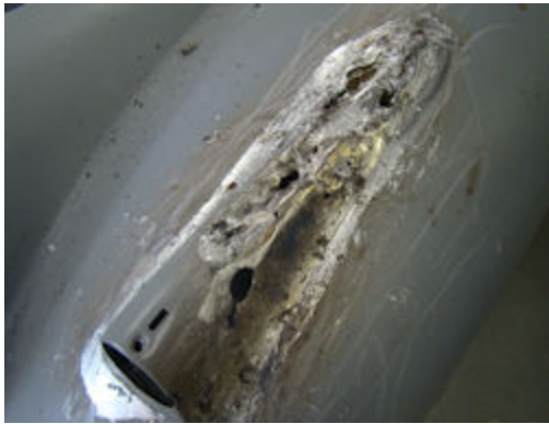
Both marker lamp housings will be replaced
