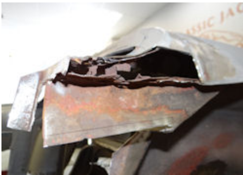
Top of driver's B pillar requires extensive surgery
