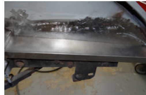
Replacement panels are fabricated and trial fitted
