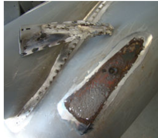
Sheet metal beneath marker lamp housings badly rusted
