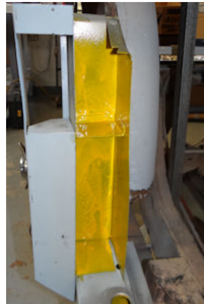
Wurth Body Wax applied to inner B pillar
