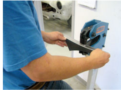
Using the shrinker/stretcher to produce the desired shape
