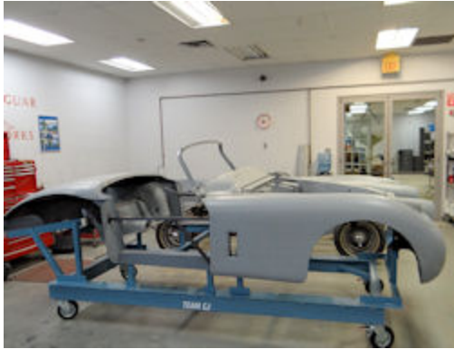
The body restoration and paint will be completed on the frame jig
