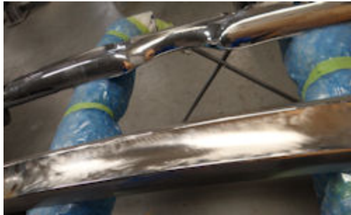
Bumpers and overriders have had 54 years worth of dents hammered out!
