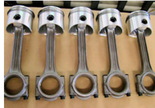
Team CJ forged pistons assembled to rods
