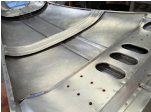
Aluminum bonnet was stripped by hand
