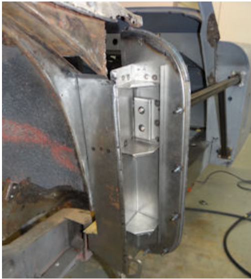
Trial fitting B pillar and door shut face panel
