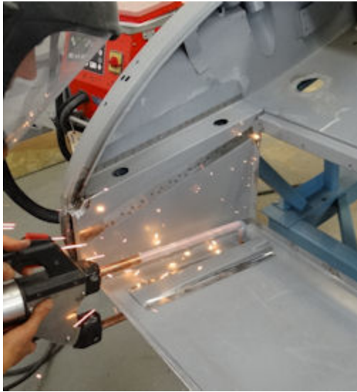
Jake spot welding boot floor braces in place
