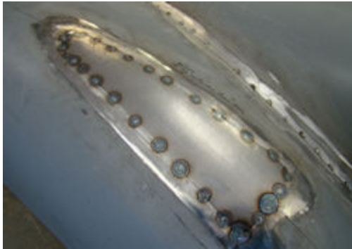
The RH sidelamp repair panel is tack welded in position...
