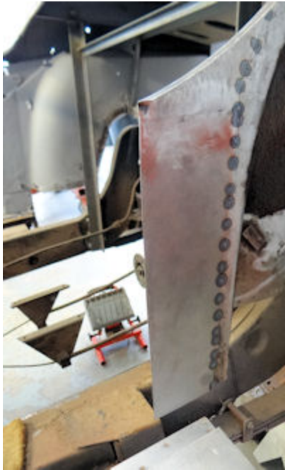
Side panel tack welded in place
