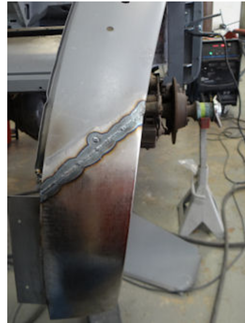
Then the repair seam is TIG welded
