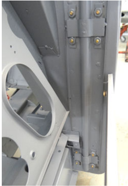
Hinge plates reinstalled after door frame shut face panels were repaired
