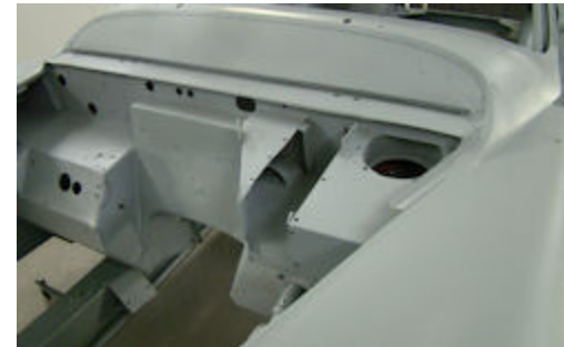
Firewall is in good shape
