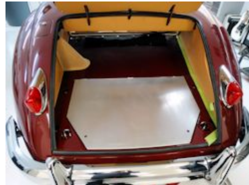
Trial fitting the new panel
