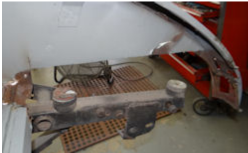
The boot compartment requires extensive rust repairs
