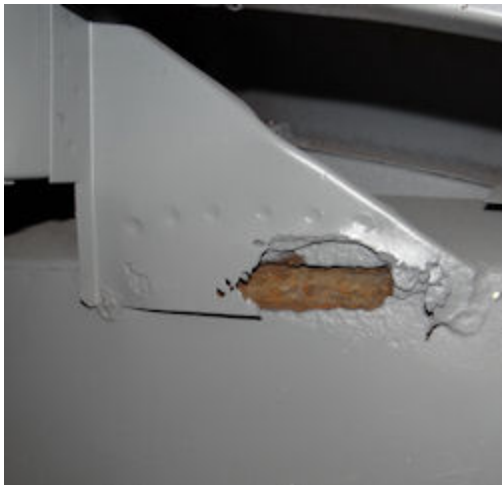
Inner rear cowl support the last rust in the entire car
