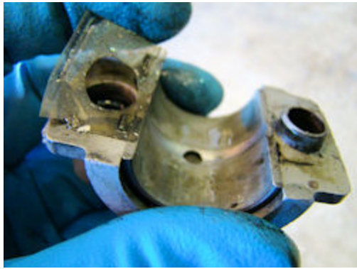
Cam caps were shimmed. Cam saddles will have to be align honed
