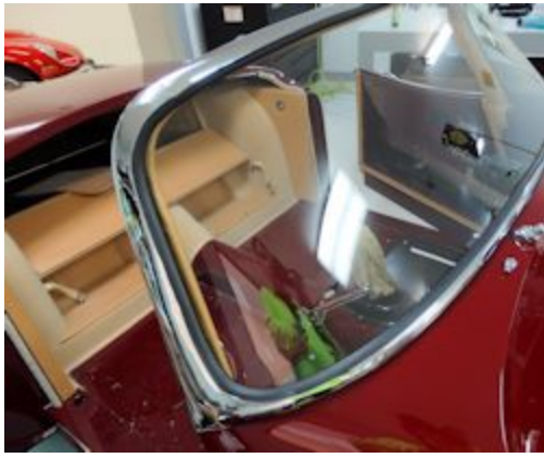
New Triplex screen installed
