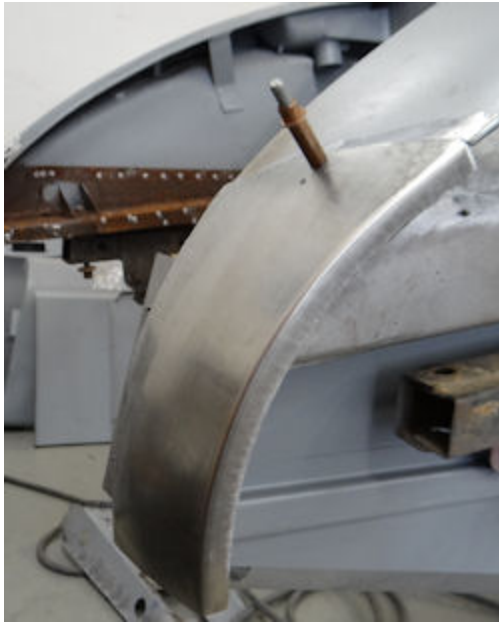
New panel matches the shape and countour of the original perfectly
