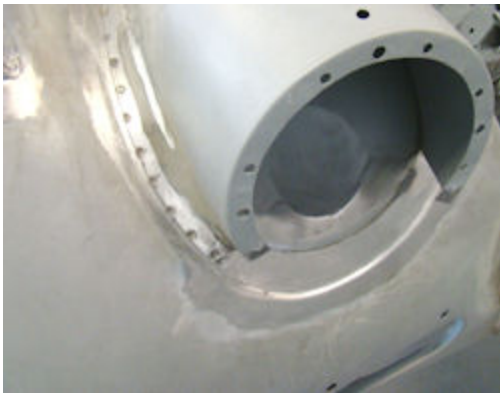
Rusted area cut away from right hand pod
