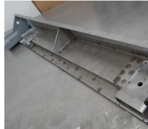
New LH rocker panel ready to install
