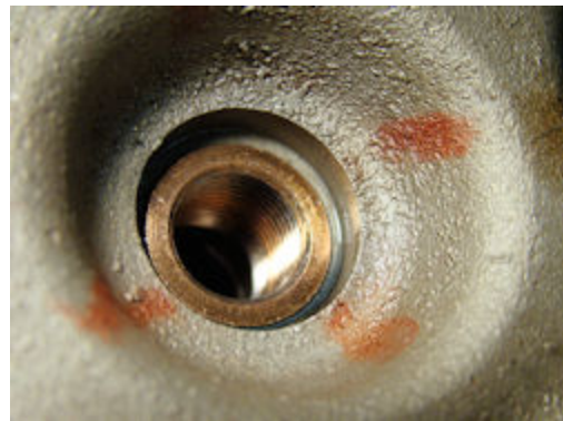
New spark plug inserts were required
