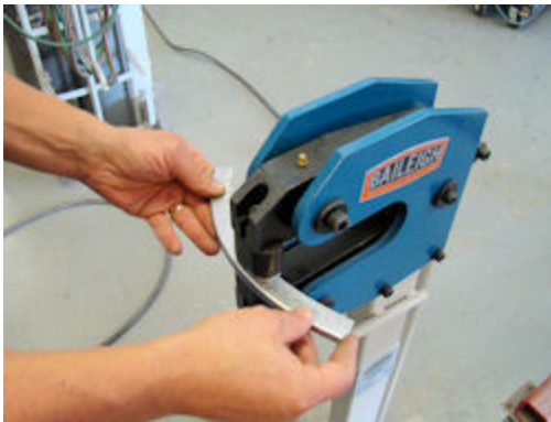
Making repair panel for headlamp mounting lip
