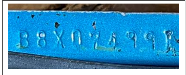
Factory correct secondary VIN of deck lid seal lip
