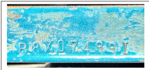
Factory correct primary VIN on radiator core support
