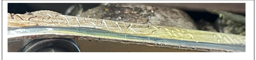
Factory correct secondary VIN of deck lid seal lip
