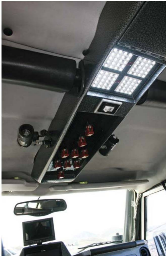
The handmade overhead console features LED lights and even red map light spots lifted from an F-16.
