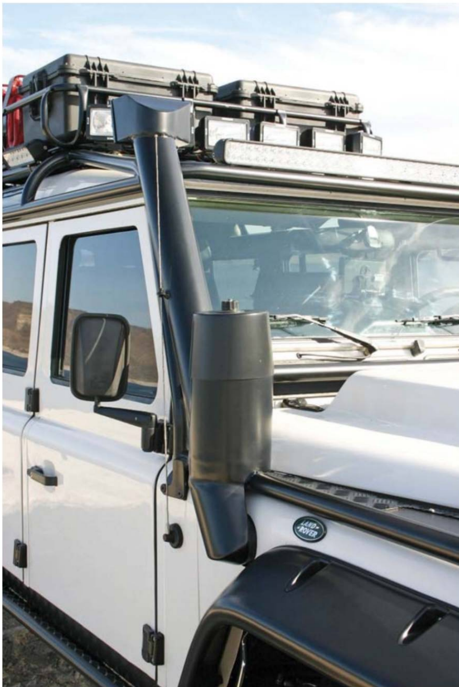
The engine breathes through a custom snorkel and air filter setup mounted on the outside of the rig.
