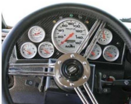
A full complement of Auto Meter Gauges is mounted in the custom dash. The Ranger Rover steering wheel came from England.
