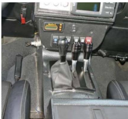
The Atlas transfer case allows for twin shifters, In and Out and High and Low Range actuators.
