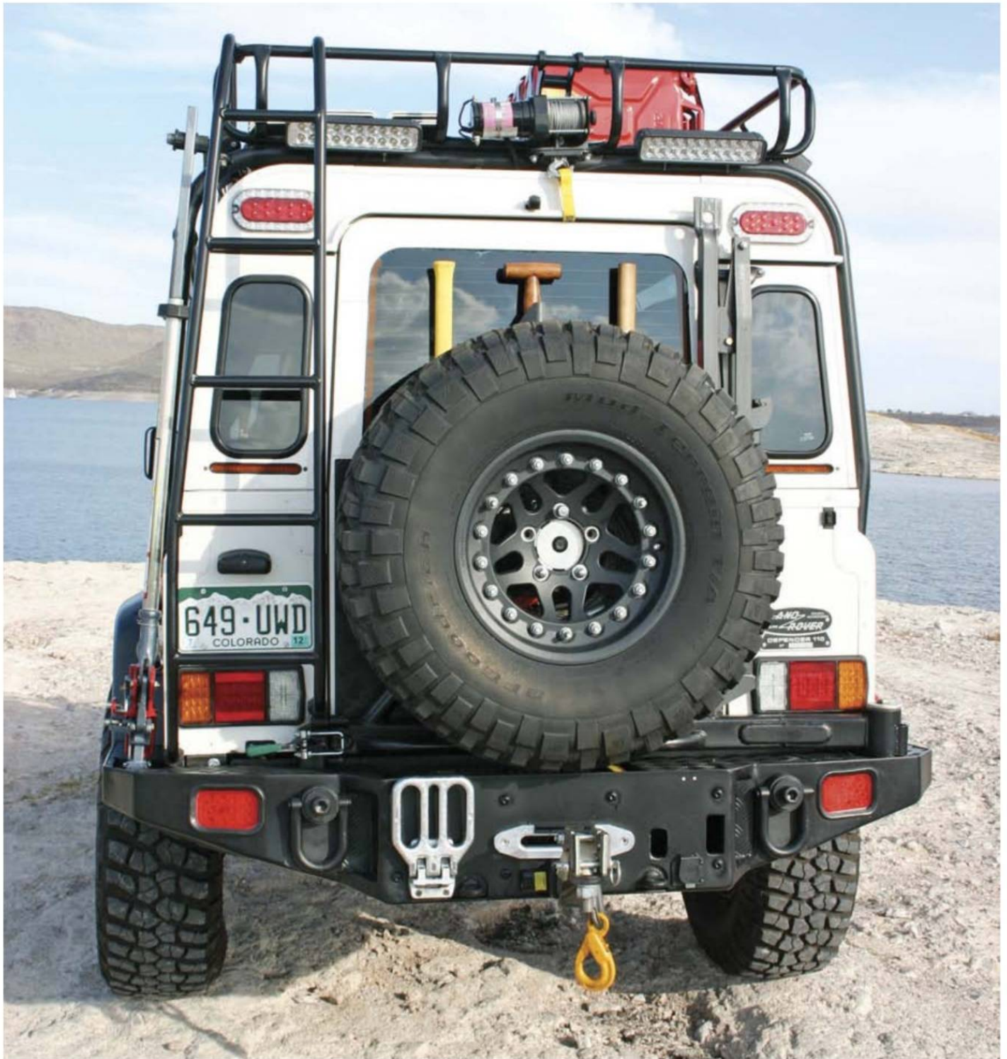
Out back, there are two winches, including one for loading cargo up on the roof rack, a fold-down step, ladder, 10,000-pound winch in the bumper and a swing-out tire carrier that hides a land anchor and hand tools.
