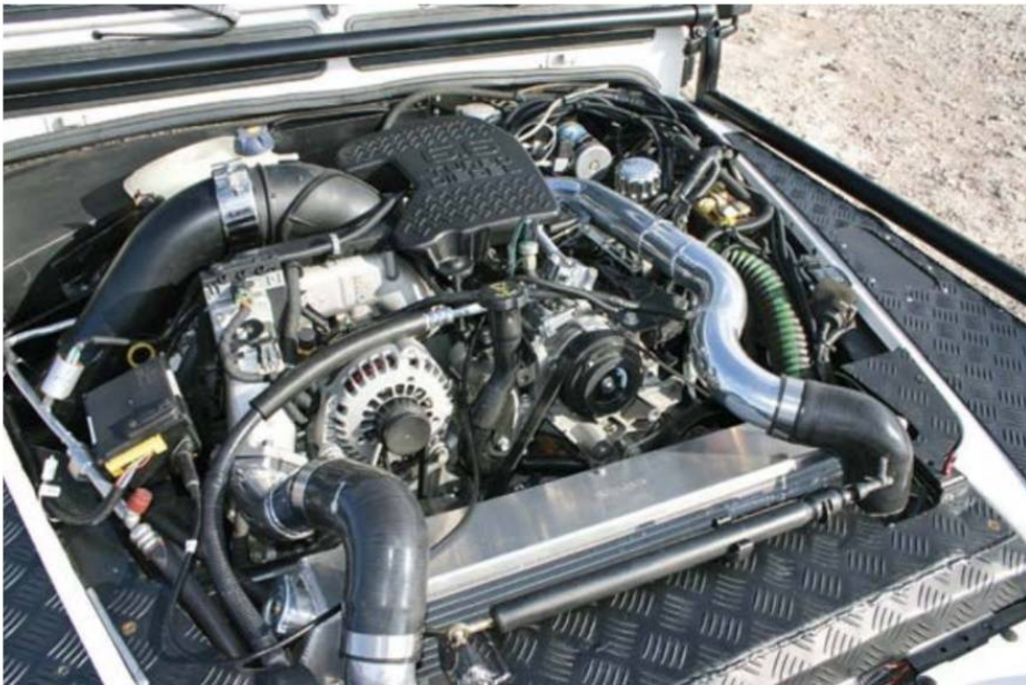
An LBZ Duramax, complete with the Allison automatic, is shoehorned into the narrow confines of the Defender's engine bay. You can see the custom plumbing for the Ron Davis intercooler that sits directly in front of one of his custom radiators.
