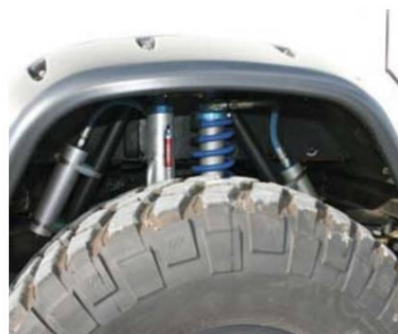
The truck features a Trick race-quality King coilover. A remote reservoir suspension provides plenty of travel and great ride quality.
