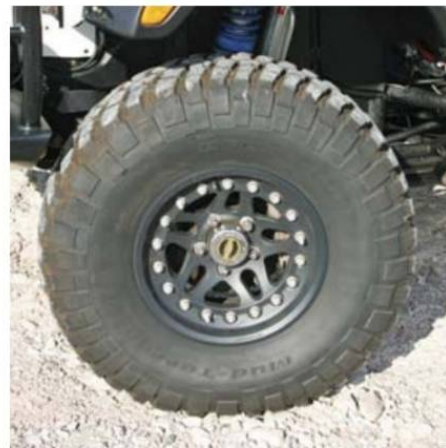
Rolling stock consists of 37-inch BFG KM2s wrapped around 17x10-inch Hutchison Rock Crawler wheels. Each axle also has a set of Warn hubs.
