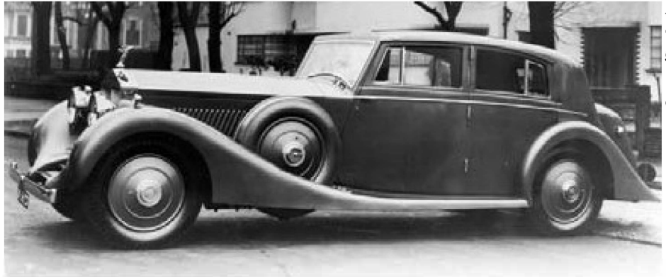
1929 Phantom II 32WJ delivered in December 1937 via Southern with this Coachcraft "Special" saloon body. It has the replacement hood for the original narrow riveted type. A most impressive car. Phantom I 80OR was similarly bodied for Malcolm Campbell Ltd.
