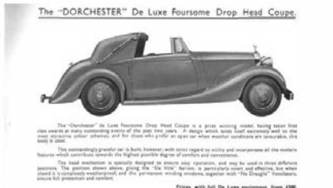
The "Dorchester" three-position coupe by Coachcraft was perhaps the most desirable of all Southern's offerings. The top cant rails, however, were detachable rather than hinged and thus not as advanced as other systems. The top was not powered. The hood sides no longer had louvers in most cases and the car looked much smoother all round.
