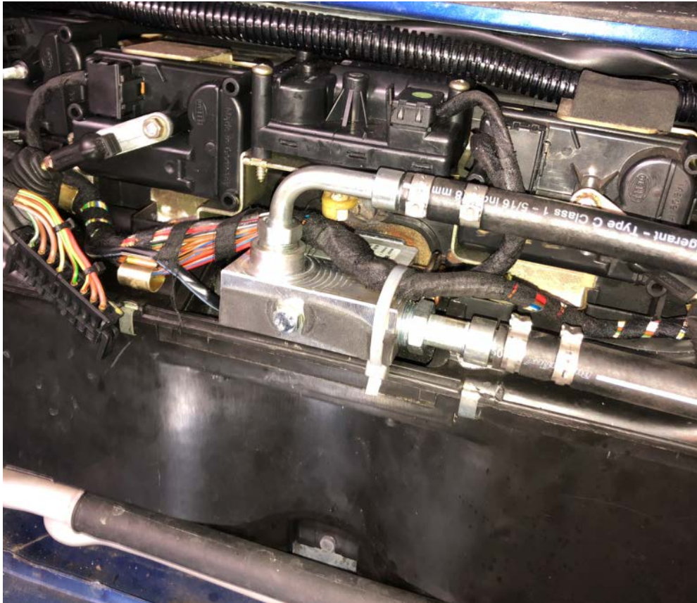
Figure 2 - Adapter block fitted. cable tie holding wiring loom away from servo arm.
