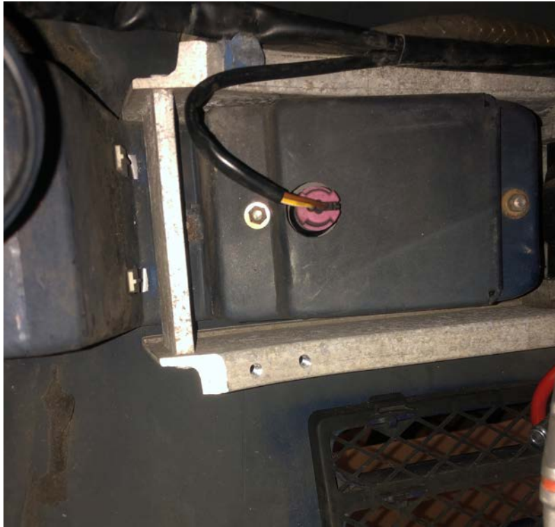
Figure 11 - Drill and tap 2 x M6 holes in bumper support for front condenser bracket.
