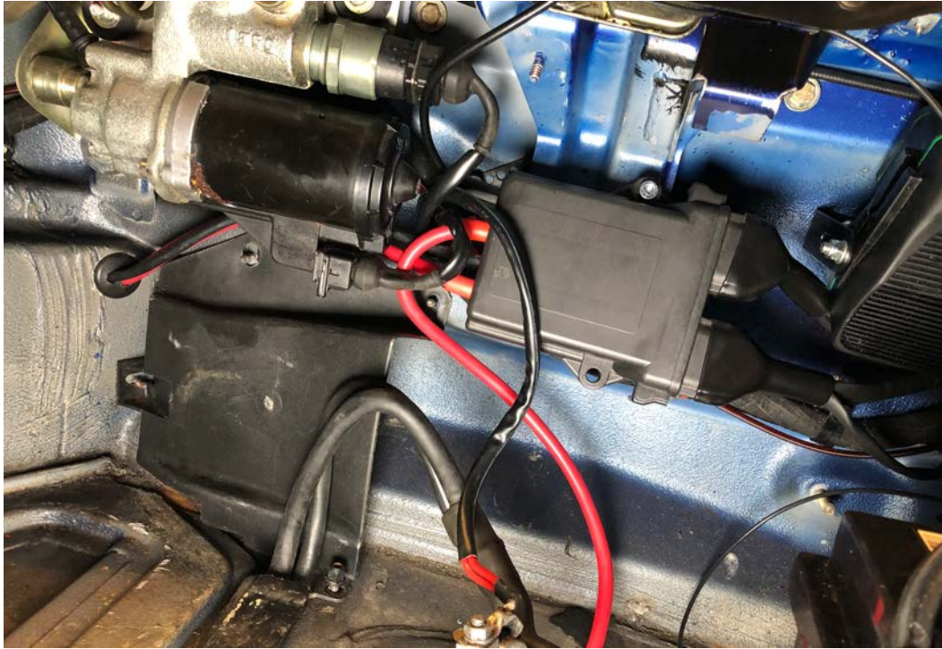
Figure 7 – Hole for heavy red wire, ECU control cable and fan cable on left. ECU can be mounted on front panel.
