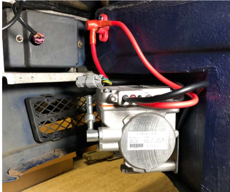
Figure 8 - ECU red wire coming through grommet and attaching to compressor +ve at power post.
