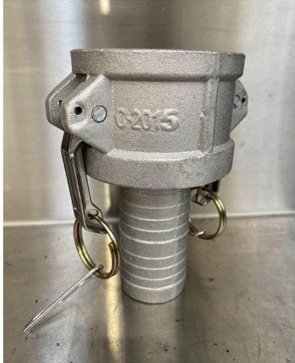
**Note:** Example of the required adaptor for connecting the deadman to the fuel delivery hose.
