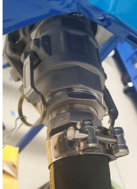
**Note:** Example of the required adaptor for connecting the deadman to the fuel delivery hose.
