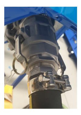
Note: Example of the required adaptor for connecting the deadman to the fuel delivery hose.
