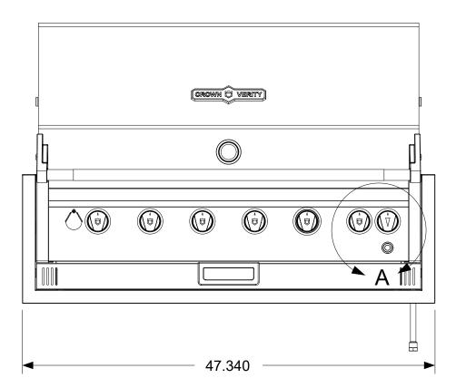
The dimensions shown are the actual physical dimensions of the grill. Additional clearances to cabinetry are dependent on the tolerances of the cut-out. The suggested cut-out dimensions are listed in the chart below but these dimensions can be reduced if the tolerances are controlled.
