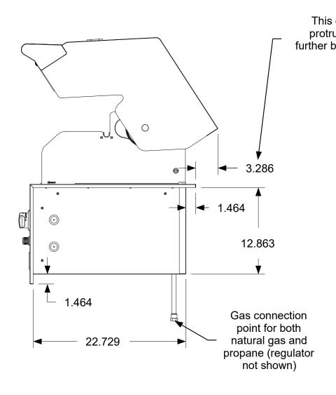
This dimension is the furthest point the dome protrudes back as it opens. It is 3.286 inches further back than the rear flange of the cabinet shell.
