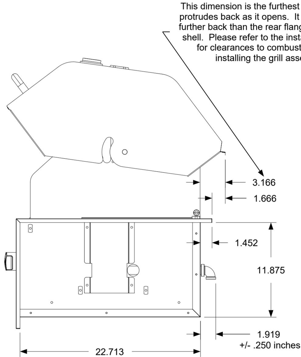
Dimensions shown are actual dimensions. Please refer to the installation manual for additional clearances and clearances to combustibles
