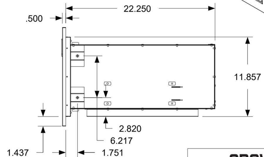
Dimensions shown are the actual physical dimensions. Additional clearances to the cabinetry are dependent on the tolerances of the cut-out. The suggested cut-out dimensions are listed in the chart below but these dimensions can be reduced if the tolerances are controlled. Please refer to the product manual for installation instructions.
