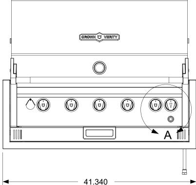
The dimensions shown are the actual physical dimensions of the grill. Additional clearances to cabinetry are dependent on the tolerances of the cut-out. The suggested cut-out dimensions are listed in the chart below but these dimensions can be reduced if the tolerances are controlled.
