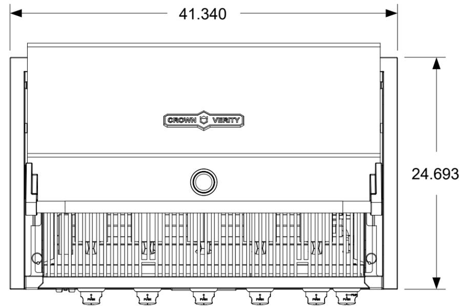
The dimensions shown are the actual physical dimensions of the grill. Additional clearances to cabinetry are dependent on the tolerances of the cut-out. The suggested cut-out dimensions for the insulated jacket option are listed in the chart below but these dimensions can be reduced if the tolerances are controlled.
