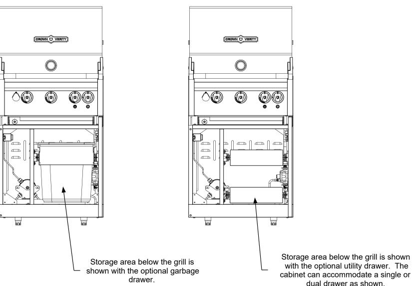
with the optional utility drawer. The cabinet can accommodate a single or dual drawer as shown.
