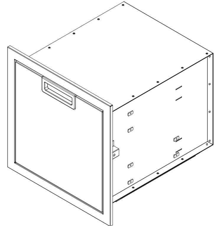
Door shown with righthand mounting option. Door hardware can be switched for a lefthand mount
