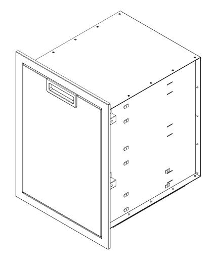
Door shown with righthand mounting option. Door hardware can be switched for a lefthand mount
