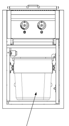
Storage are below the side burner is shown with the optional utility drawer. The cabinet can accommodate a single or dual drawer as shown
