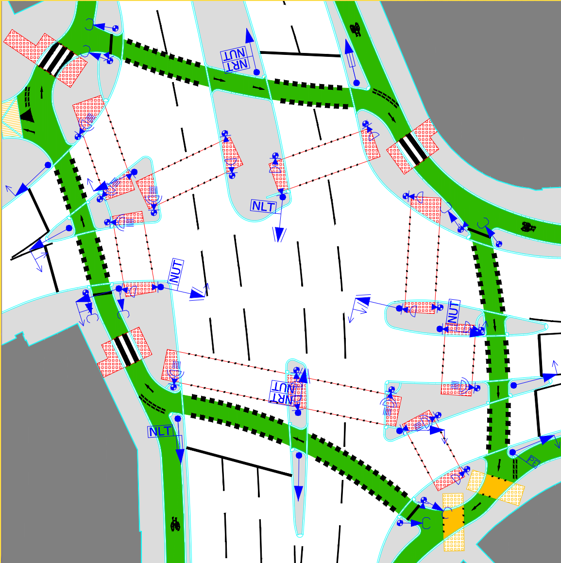
Figure 7b: Cyclops with walk-with-traffic pedestrian phases
