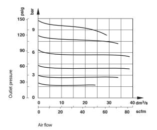
Inlet pressure: 7 bar (101 psi) Port size: 1/4", 40 µm element
