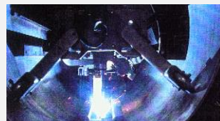
AZZ/Aquilex uses automated weld heads for precision, in-pipe operations
