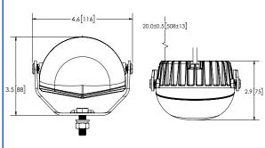
**Models** PART NO. VDC **LENS COLOR IFD COLOR LUMENS** AMPS WATTS EW2030R 12-80 Clear R 100 1.04 13.3 R 156 5.9 EW2031R 12-80 Clear 1.21
