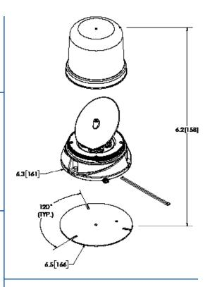
45° angled reflector driven by a quiet brushless magnetic drive system provides an exceptional warning beam without compromising reliability Eight high intensity, 3-watt LEDs combined with a unique TIR optic project light onto the reflector to provide SAE Class I light output
