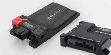
SIB & Switch Node Computer Control Network
